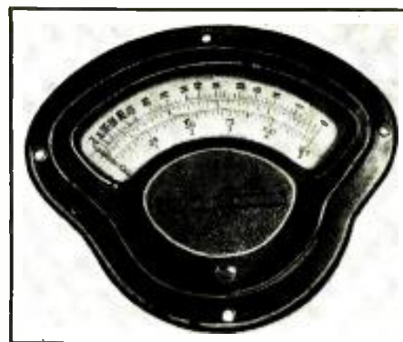
Fig. A. The meter—a current-indicating device.
