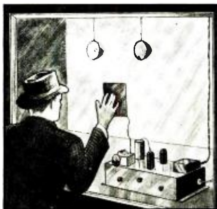
Fig. A. The completed electronic relay system in operation. A movement of the hand controls the window lights.
